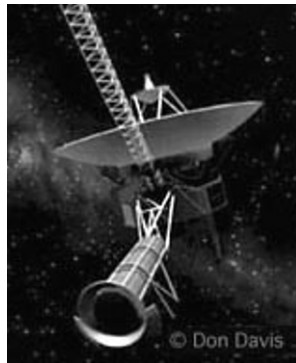
Fig. 3.1. One of the twin Voyagers , viewed from the end of its power supply boom. The science boom, not visible here, extends out the opposite side. Adapted from animation cell © Don Davis, reproduced by permission.
