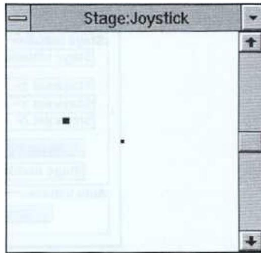
The stage Move window comprises a square area which represents the XY co-ordinate space of the stage together with a scroll bar on the right hand side which is used for stage Z control.
