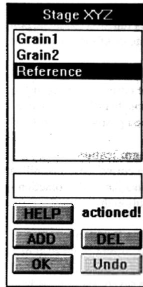
To indicate if the stage is currently positioned at the highlighted entry the legend "actioned!" will be displayed when this is the case.
