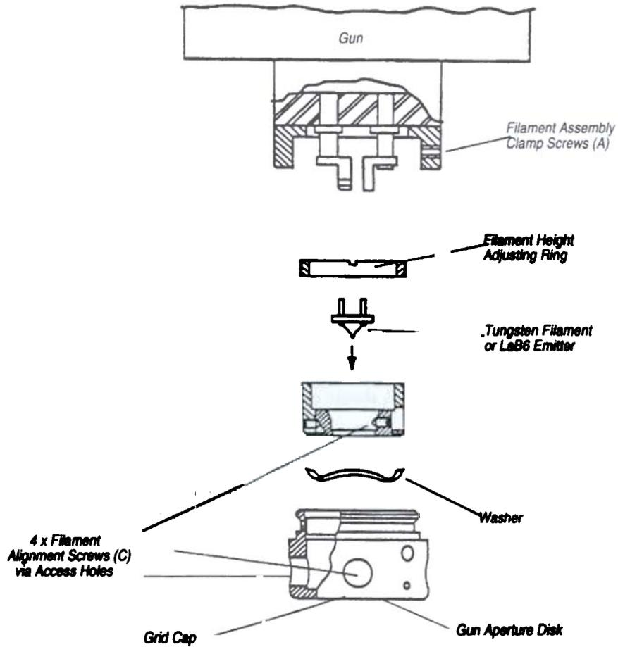
Figure 5 Firing Unit Assembly
