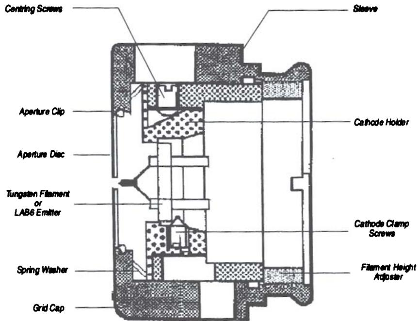
Figure 6 Cross Section of Firing Unit
