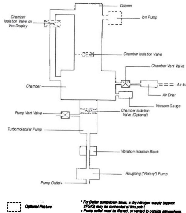
Figure 8 Identification of Isolation Valves
