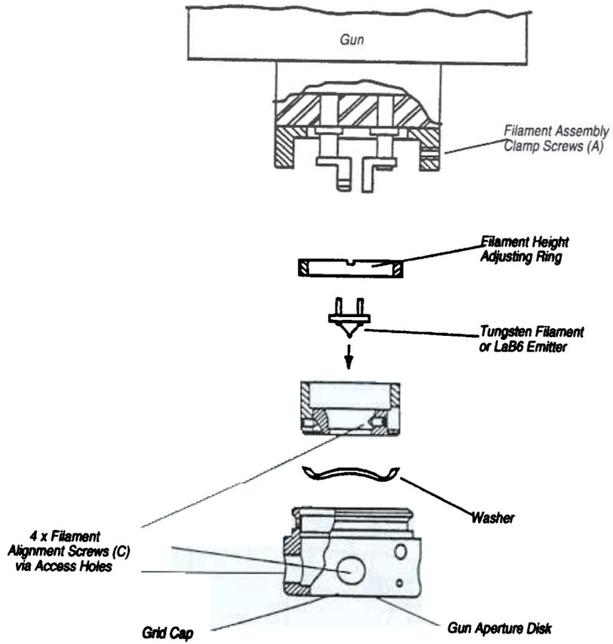
Figure 5.2 The Firing Unit
