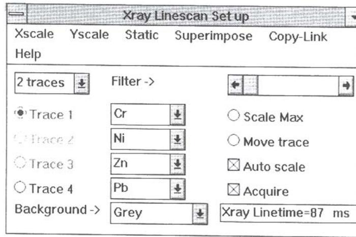
The **Xray Linescan control window** may be displayed by clicking the right mouse button over the profile window.
