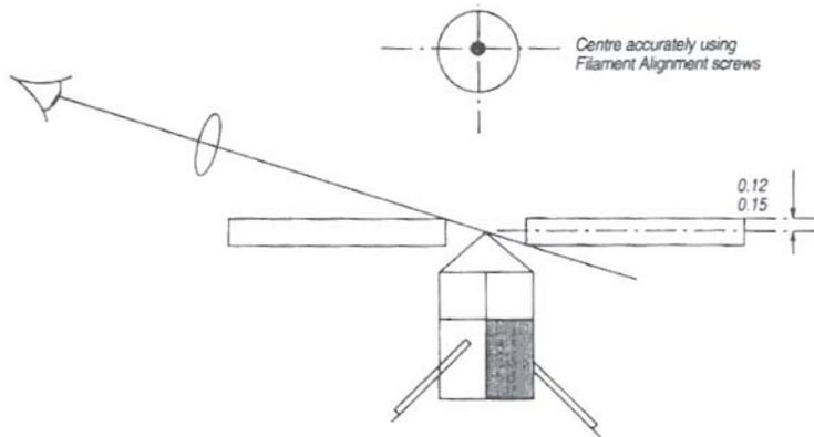
Figure 7 Lab<sub>6</sub> Cathode Height Setting
