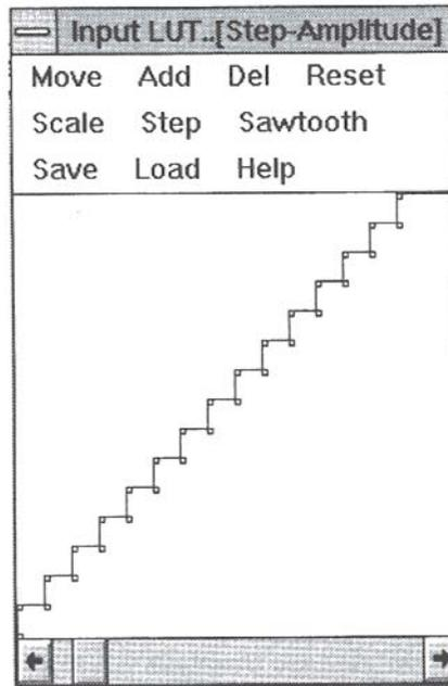
The amplitude, period and offset of the steps may be selected and adjusted using the scrollbar at the bottom of the window. The points generated may be individually moved, deleted etc.
