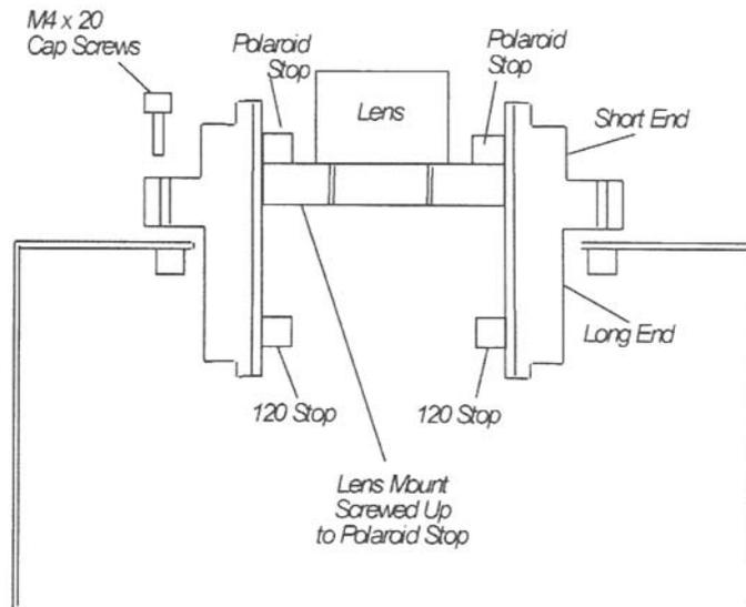
**Figure 3 Polaroid Camera Lens Mounting**
