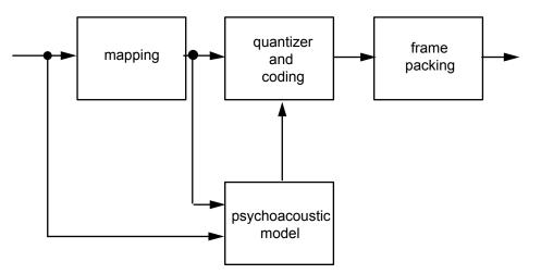
Figure I-1 Sketch of a basic encoder
