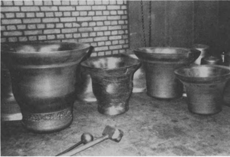
Fig. 21.11. Two new major-third bells (left) compared to conventional (minor-third) bells with the same pitches.
