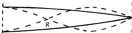
Fig. 15.3. Positioning of a register hole in a cylindrical instrument, such as the clarinet. The curves show pressure standing waves for the first and second modes of the pipe.
