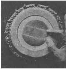
Fig. 18.14. Method used to excite the mode in Fig. 18.13(c). Two fingers damp the membrane at the two nodes, and a third finger strikes it at a point 90° away (from Raman, 1934).
