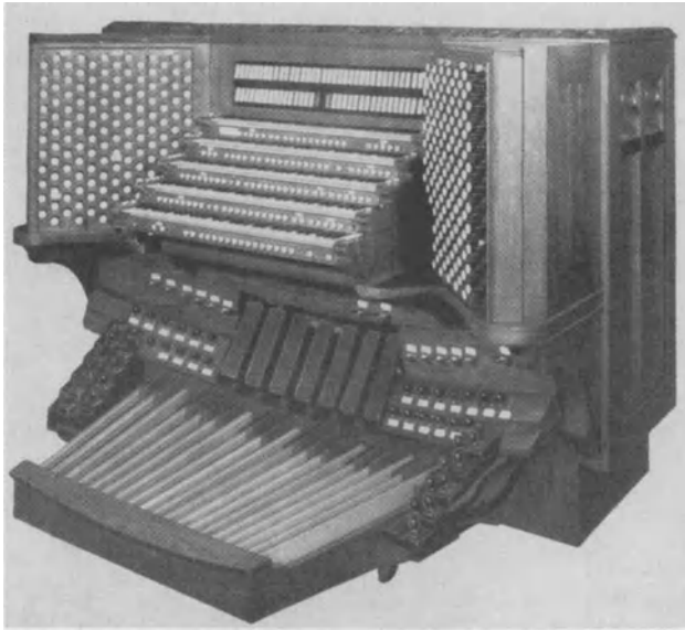
Fig. 17.5. The console of a large organ. The drawstops are mounted on the wings, buttons under each keyboard control groups of stops, usually in an adjustable manner, and their functions are duplicated by toe studs. The inclined flat pedals control the opening of the various swell shutters (Aeolian–Skinner).
