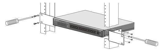
Figure 4-1. Attaching Mounting Brackets
