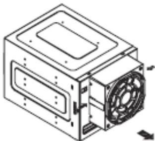
**Figure D-6: Removing the Exhaust Fan**
