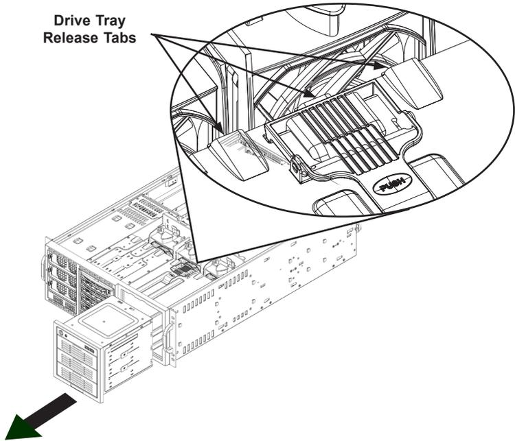
**Figure 5-10: Removing the Drive Bay**
