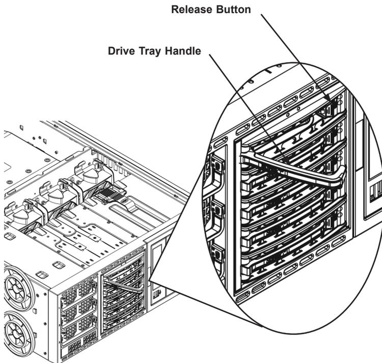
Figure 5-13: Install Hard Drives
