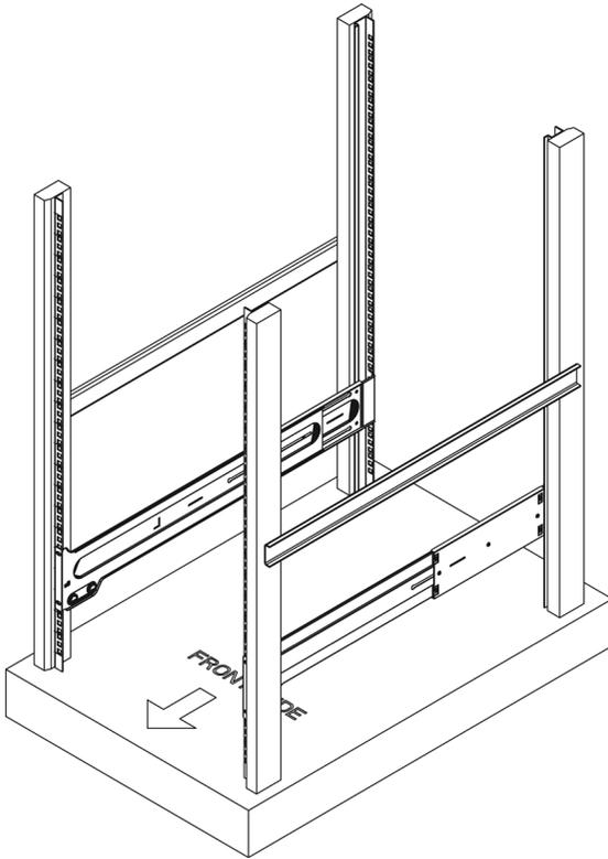
**Figure 6-6. Installing the Rack Rails**
