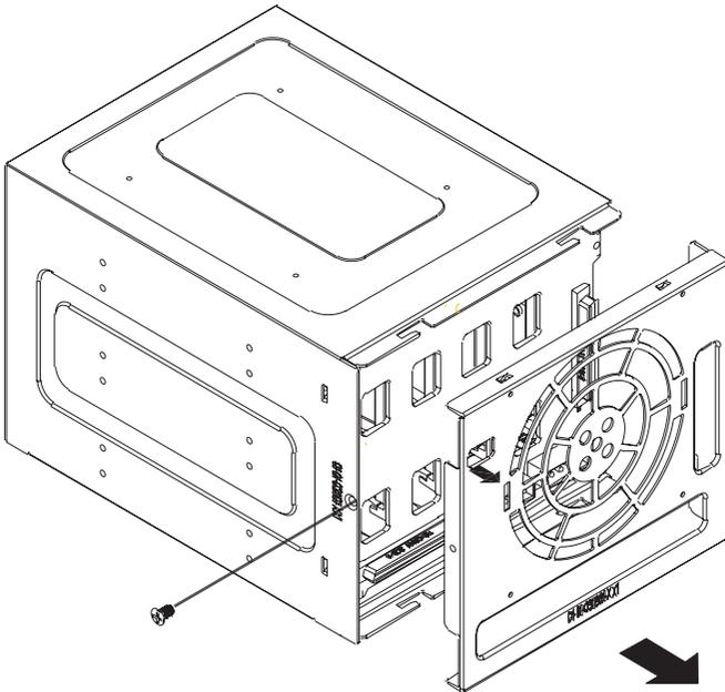
**Figure C-7: Removing Mobile Rack Fan**
