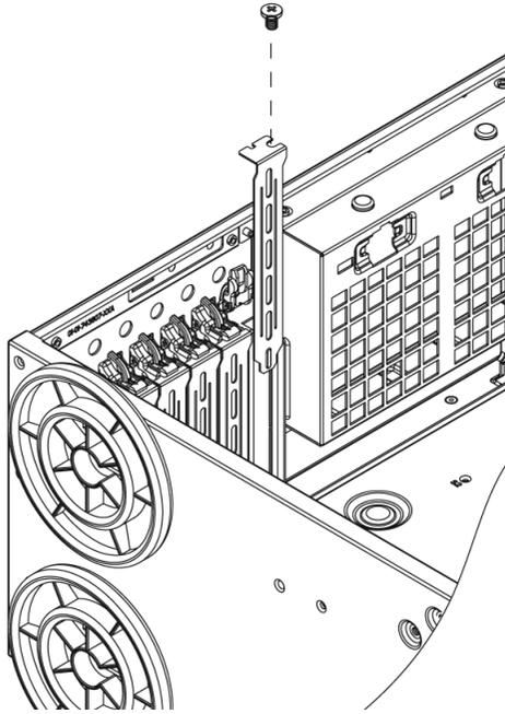
**Figure 5-20: Remove PCI Card Slot Guard**
