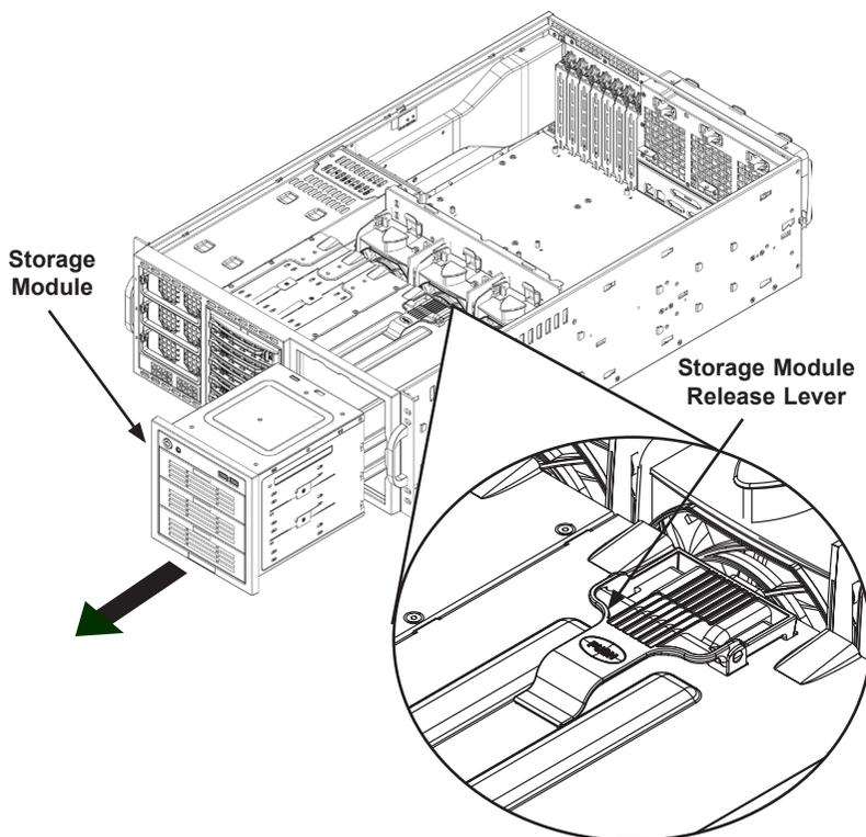
**Figure 5-4: Remove the Storage Module**
