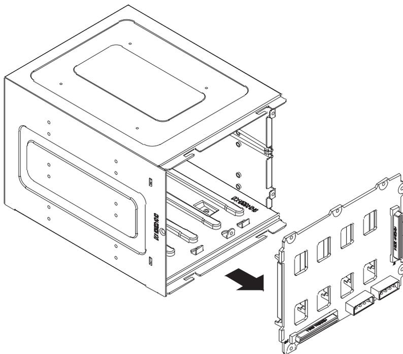
**Figure C-8: Removing Mobile Rack Fan**
