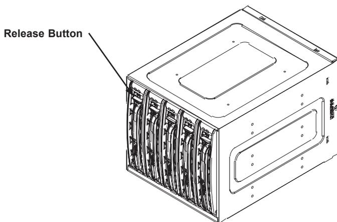
**Figure D-3: Hot-Swappable Drive Release Button**
