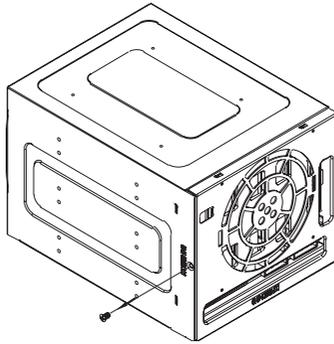
2. Pull out the rear bracket (as shown below:)
