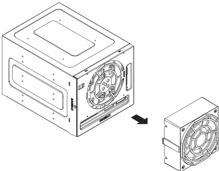
**Figure C-6: Removing Mobile Rack Fan**
