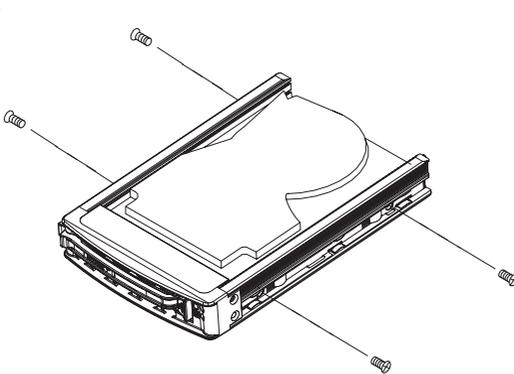
**Figure 5-15: Installing the Hard Drive**
