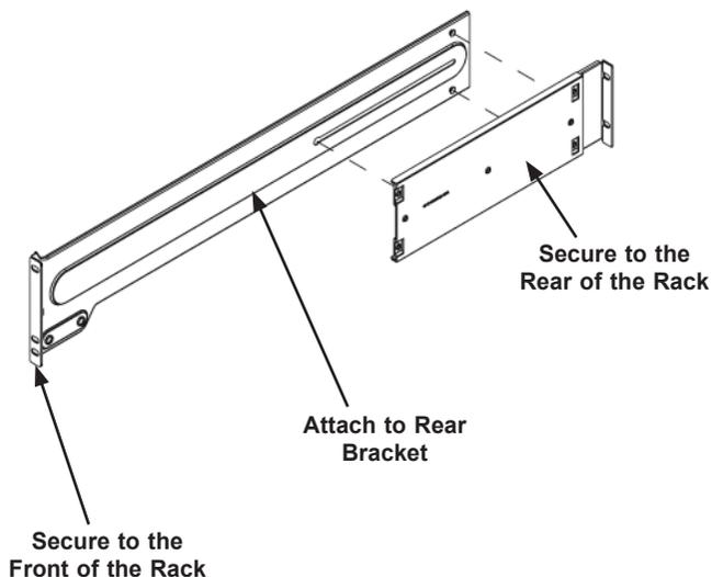
**Figure 6-5: Assembling the Outer Rails**
