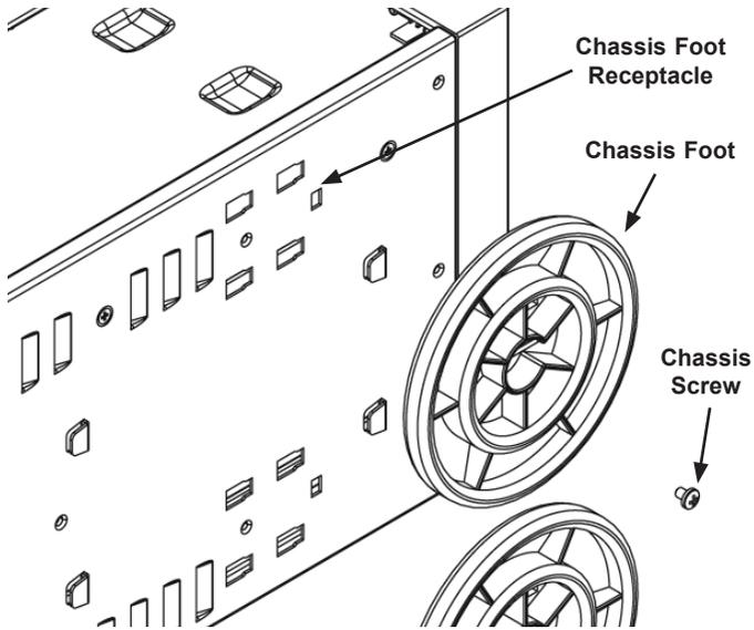
**Figure 6-9: Placing Chassis Feet**
