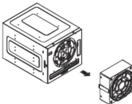
**Figure D-7: Pulling Off the Exhaust Fan**
