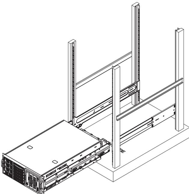
**Figure 6-7: Installing the Chassis into a Rack**
