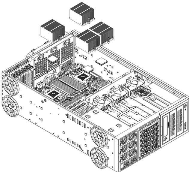
**Figure 5-18: Installing Heatsinks**
