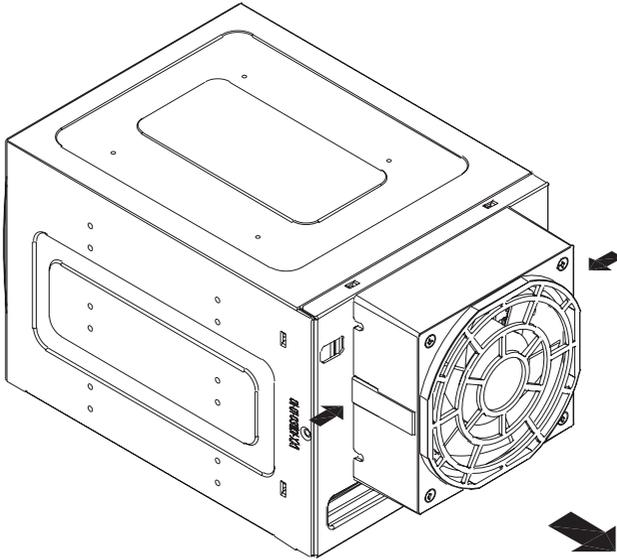
**Figure C-5: Removing Mobile Rack Fan**
