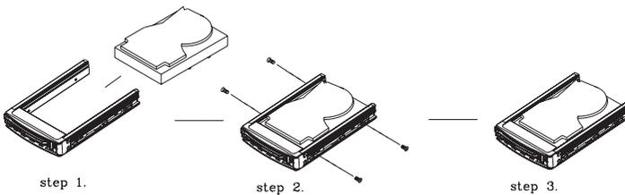
**Figure D-5: Mounting Drives**
