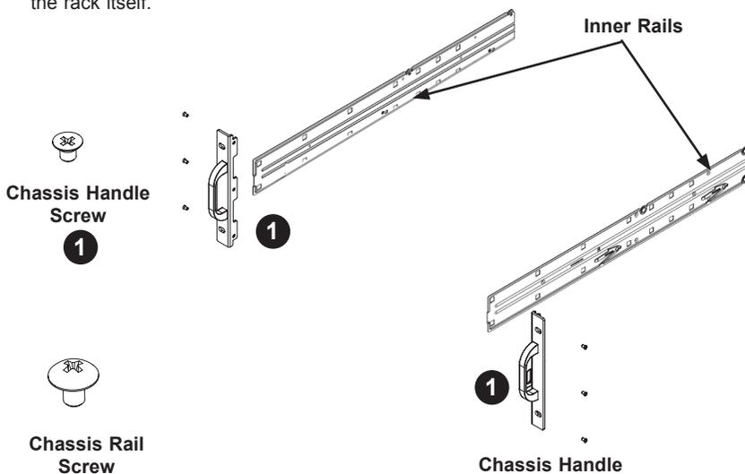
**Figure 6-2: Identifying the Inner Rails and Chassis Handles**
