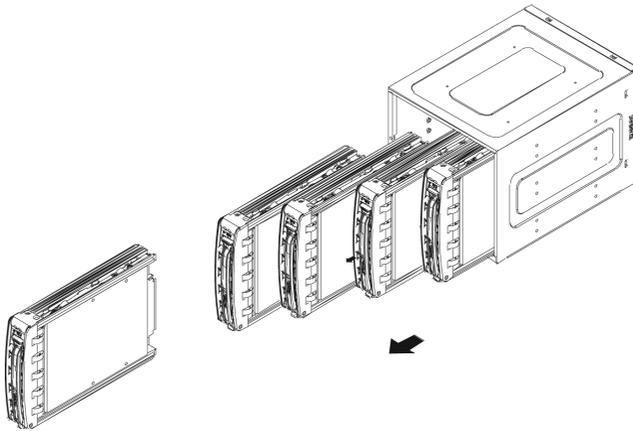
**Figure D-4: Removing Drives**
