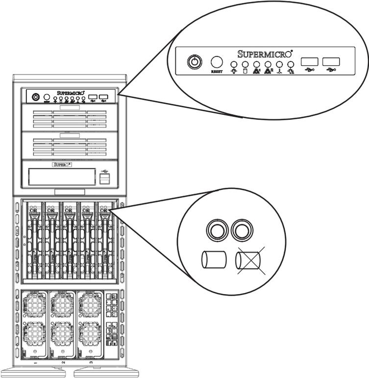
Figure 4-1: Front LEDs
