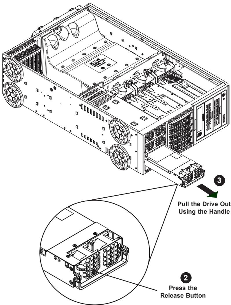
Figure 5-25: Removing a Power Supply
