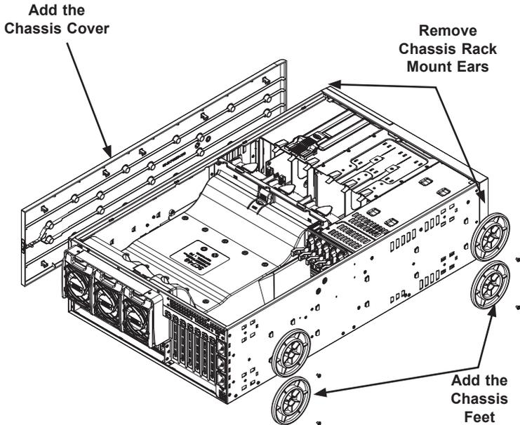
Figure 6-8: Adding Chassis Feet and Top Cover
