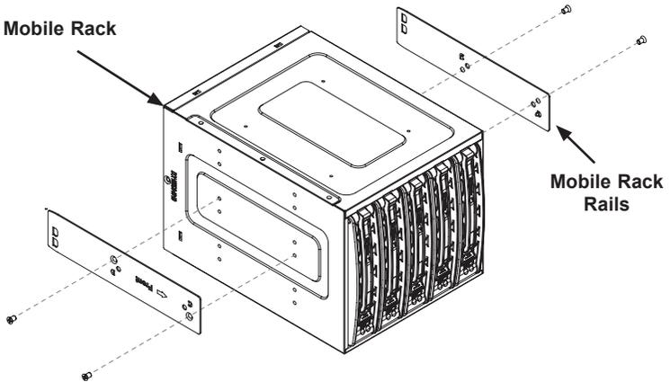
Figure 5-12: Add Storage Module Rails to the Mobile Rack
