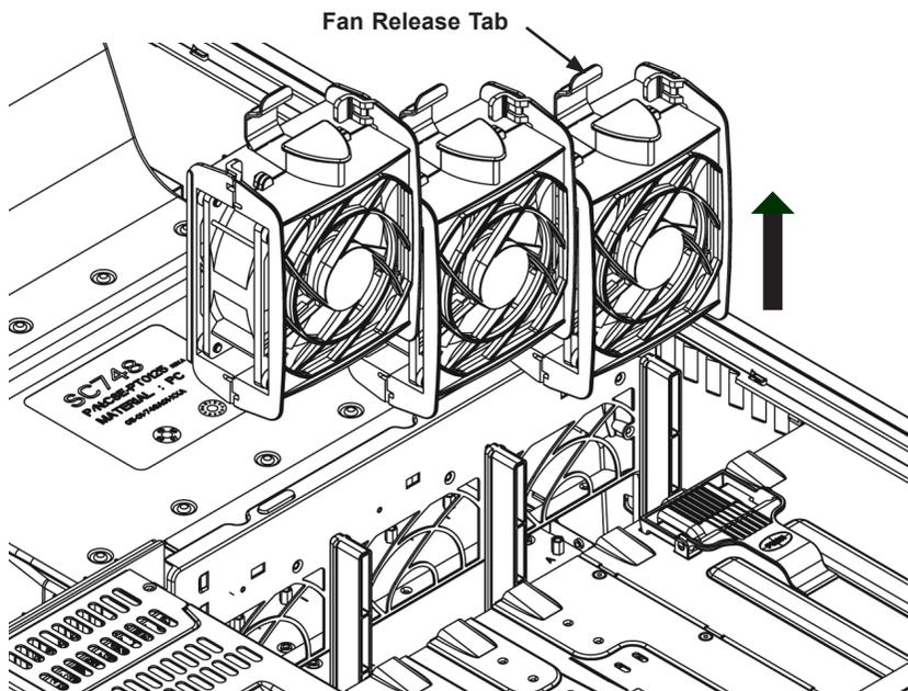
Figure 5-23: Front Chassis Fans
