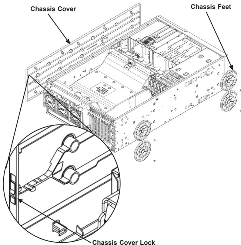
Figure 6-1: Remove Feet and Chassis Top Cover
