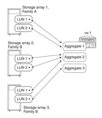
In Example 2, one storage array is from Family A and two storage arrays are from Family B. The LUNs from the Family A storage array cannot be assigned to the same aggregate as the LUNs from a Family B storage array because they are in a different family. However, LUN 1 of storage array 3 can be assigned to aggregate 2, which also contains LUNs from storage array 2, because the two storage arrays are in the same family.
