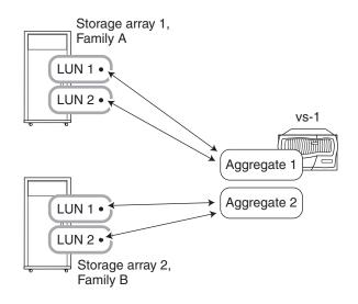
**Example 2:** LUNs from the same storage array family can be mixed in an aggregate but LUNs from a different storage array family (or different vendor) cannot be mixed.
