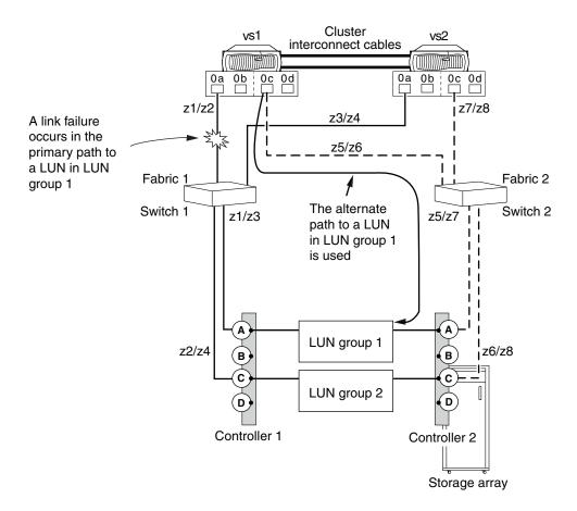
Failover in this example with two LUN groups works the same way as in the first failure scenario (assuming the primary path from vs1 to a LUN in LUN group 1 is through vs1's FC initiator port 0a). If a failure occurs in the link between vs1's FC initiator port 0a and Switch 1. Data ONTAP automatically switches to the alternate path through vs1's FC initiator port 0c, which enables vs1 to access the LUN in LUN group 1 through Switch 2 and then through the storage array's Controller 2 port A.
