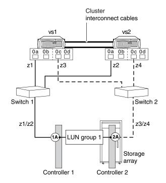
**Applicability of this configuration:** This configuration, with one 2-port array LUN group, works with all storage arrays for all Data ONTAP releases.
