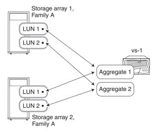
Example 3 is not supported if one of the storage arrays has Fibre Channel drives and the other storage array has SATA drives.
