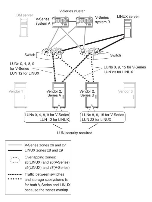
Overlapping zoning on the switch is set up as shown in the following table.
