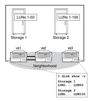
In the example, the output from the disk show -v command on all three V-Series systems shows that all three V-Series systems can see the same LUNs from Storage 1 and Storage 2. All V-Series systems in the neighborhood must be able to see the same LUNs (although in Data ONTAP only one system is assigned as the owner of the LUN).
