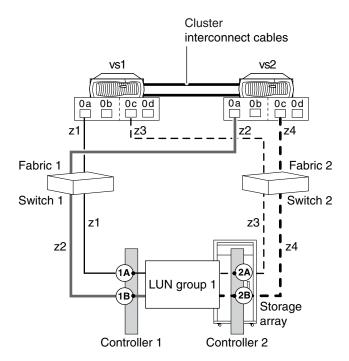
**Applicability of this configuration:** This configuration, with one 4-port array LUN group, works with all storage arrays for all Data ONTAP releases.
