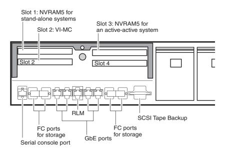
**V3070 and V3040 systems using NVRAM6:** The following illustration shows the locations of the onboard ports, PCI slots, and AC connections on all configurations of the V3070 and V3040 systems.
