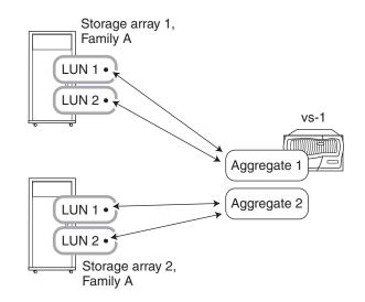
**Example 3:** Multiple aggregates, with array LUNs from the storage arrays in the same family mixed in the aggregates.
