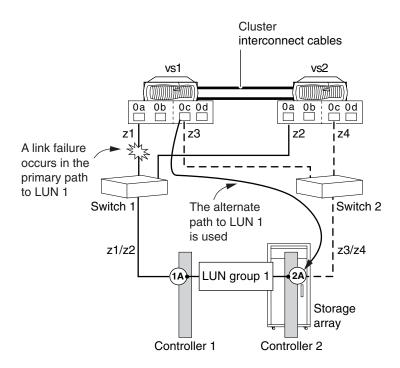
In this scenario, the primary path to LUN group 1 from vs1 is through vs1's FC initiator port 0a, to Switch 1, and then to the storage array's Controller 1 port 1A. If a failure occurs in the link between vs1 FC initiator port 0a and Switch 1 when vs1 tries to access LUN group 1, Data ONTAP automatically switches to the alternate path through vs1's FC initiator port 0c. V-Series vs1 can then access LUN group 1 through Switch 2, and then through storage array Controller 2 port 2A.
