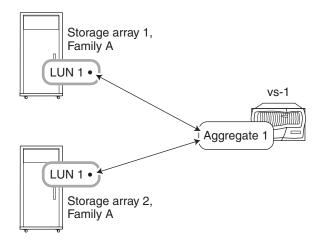
**Example 2:** Multiple aggregates, each of which contains array LUNs from a single storage array even though the storage arrays are from the same family.
