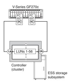
With a GF270c deployed with an ESS or a DS8xxx storage array, if one path fails, a takeover by the partner in the V-Series HA pair occurs.
