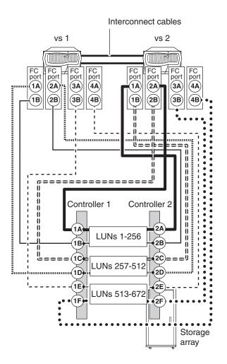
For each node in the HA pair, the same set of array LUNs must be visible on two separate adapters on the node for redundancy. Then, if one adapter fails, the array LUN group is still accessible from the other adapter on the same V-Series system. The following table summarizes the redundant paths shown in the illustration for each array LUN group for each node in the HA pair.
