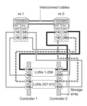
For each node in an HA pair, the same set of array LUNs must be visible on two adapters on the node for redundancy. Then, if one adapter fails, the array LUN group is still accessible from the other adapter on the same V-Series system. In the illustration, the port pair is represented by the same line type. The following table summarizes the redundant paths shown in the illustration for each array LUN group for each node in the HA pair.
