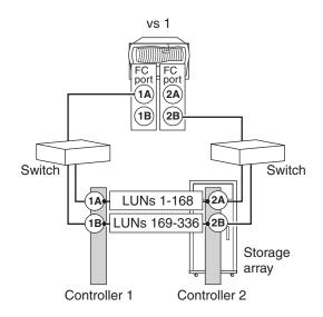
Assume that 336 array LUNs were allocated on the storage array for the V-Series systems and that the V-Series model can support 336 array LUNs. For storage arrays that support only 256 array LUNs per host group per port or 256 array LUNs per port, you must add a second port pair to handle from 257 and 336 array LUNs. You cannot just add another host group on the storage array port to increase the number of V-Series LUNs. The array LUNs are distributed equally over the port pairs.
