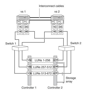
For storage arrays that support 256 array LUNs per host group per port or 256 array LUNs per port, you must have (at least) three port pairs to handle any number of array LUNs between 513 to 672.
