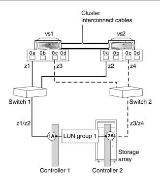
To ensure availability, use a redundant port pair on each V-Series system (that is, one connection from each adapter on a V-Series model with cards or a port from each bus for a model with onboard ports). Then, if one path from a V-Series node fails, the other path from the node is used; V-Series controller takeover does not occur.
