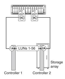
You can divide the LUNs in this configuration between the CPU modules (heads) on the GF270c if the maximum and minimum model-specific LUN counts per CPU module are met (see the V-Series *Support Matrix* for more information).
