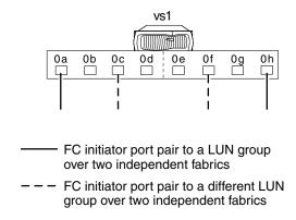
To use multiple V-Series port pairs as the illustration shows, each port in a V-Series port pair must access a different fabric.
