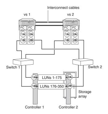
For storage array models that support 256 array LUNs per host group per port or 256 array LUNs per port, you must have at least two dedicated port pairs to handle 257 to 512 array LUNs. You cannot just add another host group on the existing port to increase the number of array LUNs for the V-Series system.
