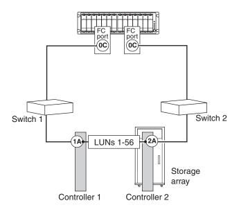
Only two ports are supported on the GF270c. Two switches are deployed for redundancy, in case one switch fails.
